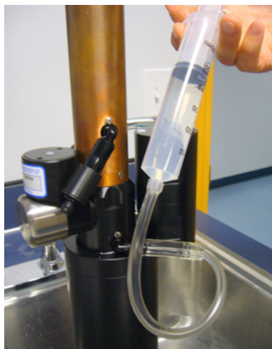
Figure 15 Triton® X-100 solution into the CT-DO
