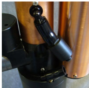
Figure 20 Tube disconnected from bottom elbow
